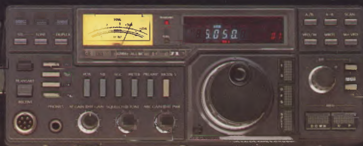
IC-471A UHF Multi-mode 430 - 450 MHz / 10 Watts
