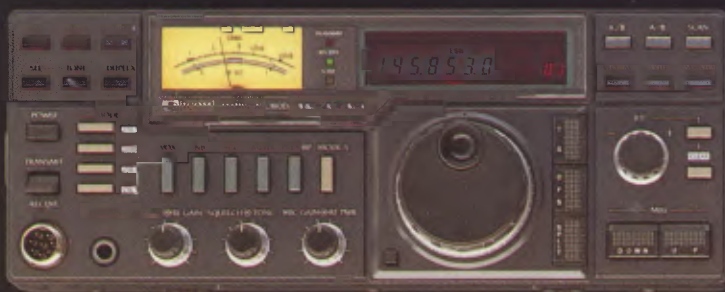
IC-271A VHF Multi-mode 2 Meter / 25 Watts
